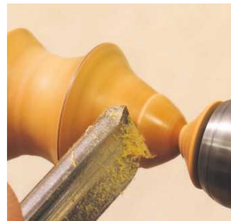
▲ Pic.33 He decided to finish the ends in a mushroom-top shape. You can take down the shape just leaving a few millimetres of timber remaining
